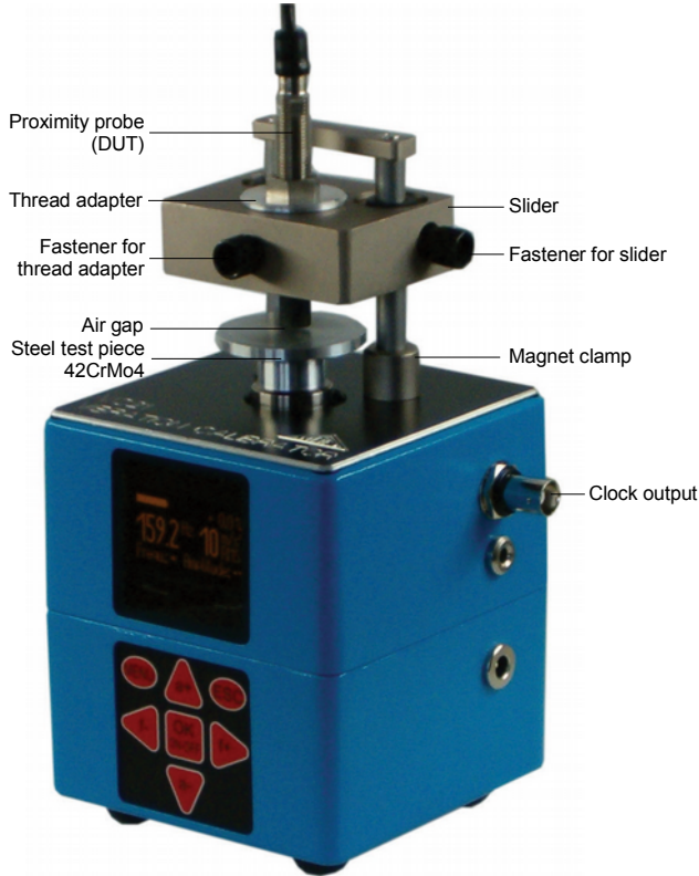
Figure 2: VC21D with clamping device for proximity probes and clock output
