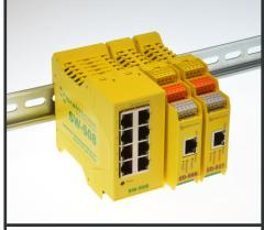
Integral DIN mount and slim design provides Ethernet connection to multiple devices
