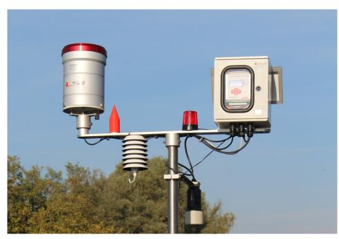
The storm front distance sensor is particularly suitable to be connected to **Alpha-Log** (DLALA0100.1) data-logger and mounted on the DYA046 bar (see figure), or fixed on the DYA032 mounting arm, to complete an **early warning** solution.
