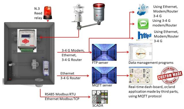
In the picture above there is a general overview of the Alpha-Log data logger data communication/management possibilities. Communication ports/device and data format (Ethernet, RS232-485 ports. HTTP, Modbus RTU/TCP, FTP MQTT protocols), power outputs and alarms by SMS are available in a single device.
