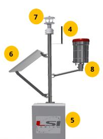
Compact weather station including data logger with solar panel and 3G modem for data communication. Ethernet, WiFi or 4G-Lte Router are alternative for data communications. The system is mounted on a H.2 m pole fixed on a concrete plinth or to walls.
