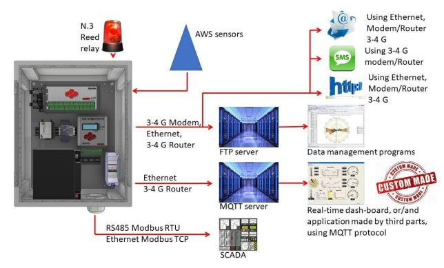
General overview of the Alpha-Log data logger data communication/management capabilities. Communication ports/device and data format (Ethernet, RS232-485 ports. HTTP, Modbus RTU/TCP, FTP, SFTP, MQTT protocols), power outputs and alarms by email and SMS are available in a single device.
