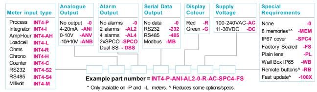
**INT4- AH** Precision Ampere-Hour or Ampere minute or Coulomb meter. Ideal for electro-plating applications. You can view the current, set alarms to dose chemicals or to shut off the process on reaching target charge.
